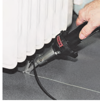
The HOT JET S is especially suited to carry out work in areas which are difficult to access.
