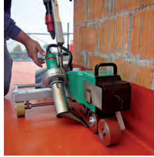
Thanks to its slim line design, welding is possible in gaps as narrow as 110 mm.
