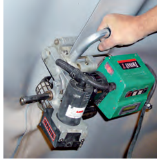
TWINNY T with convenient cross-handle at work: overhead welding in a tunnel.
